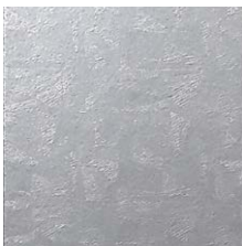
Acrylic Coated Galvalume TSR = 55%
